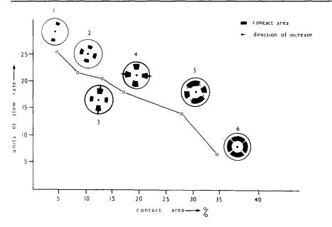
Fig. 3. Flow rate as a function of the degree of contact area.
