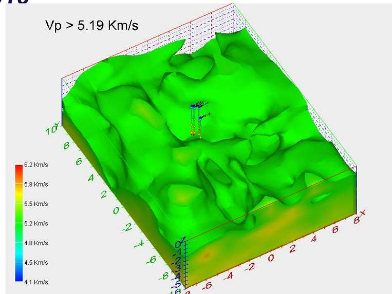
Fig.10. 3D view of Delvina anticline structure and the surrounding structures based on Passive Seismic results ( $V_p > 5.19$ ). The production wells are on top of the anticline structure.
