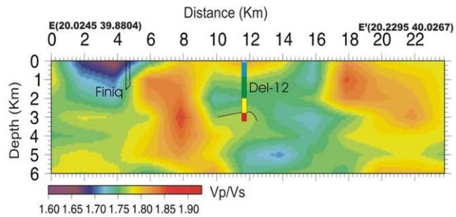
Fig.8.  $V_p/V_s$  results versus depth along EE'.
