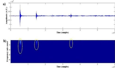
Figure 1: Example of seismic record (vertical component) a) and the corresponding image containing the polarization differences between the NS and EW records b). The recorded seismic events are indicated in red ellipses.
