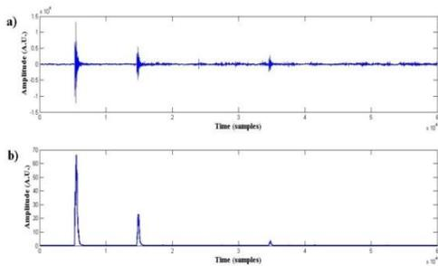
Figure 2: Example of seismic record (vertical component) a) and the corresponding proposed characteristic function b).
