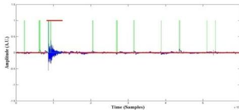
Figure 5: Example of the implementation of the proposed event detection algorithm (red dots) and the STA/LTA algorithm (green lines) on a good quality signal recorded in Silchar, India .
