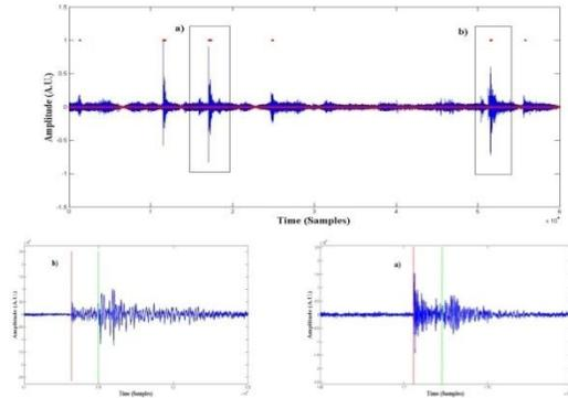
Figure 6: Example from the implementation of the proposed methodology on seismic data recorded in Kefalonia, Greece (upper plot), as well as P- and S- arrival times estimation for the selected events in the black rectangles (bottom plots).
