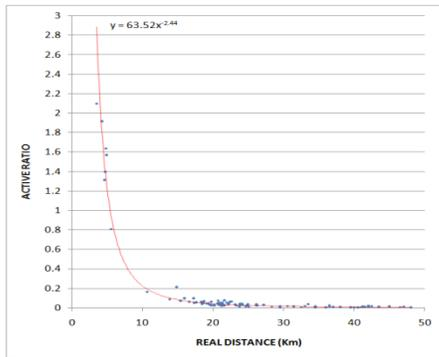
Figure 4: “Active” ratio for the above four seismic events in relation with the real distance of each hypocenter. The corresponding regression curve in red is used for a “rough” distance estimation.
