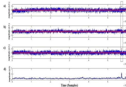
Figure 7: Example of the implementation of the proposed methodology on poor quality seismic data recorded in Delvina, Albania, during a hydraulic fracturing experiment. The 3C seismic record with the detected segment (red dots, a),b) and c) and the corresponding characteristic function d).
