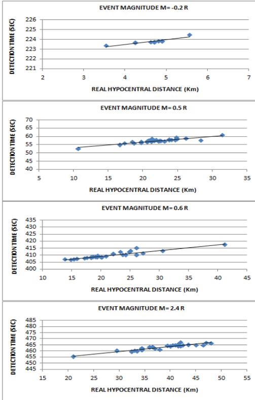
Figure 3: Detection time (time corresponds to the maximum value of characteristic function) versus the real hypocenter distances as estimated by expert analysts, for four different seismic events. The corresponding regression lines are indicated with black lines.
