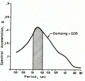
Fig.5. Mean acceleration response spectra for Knossos site.
