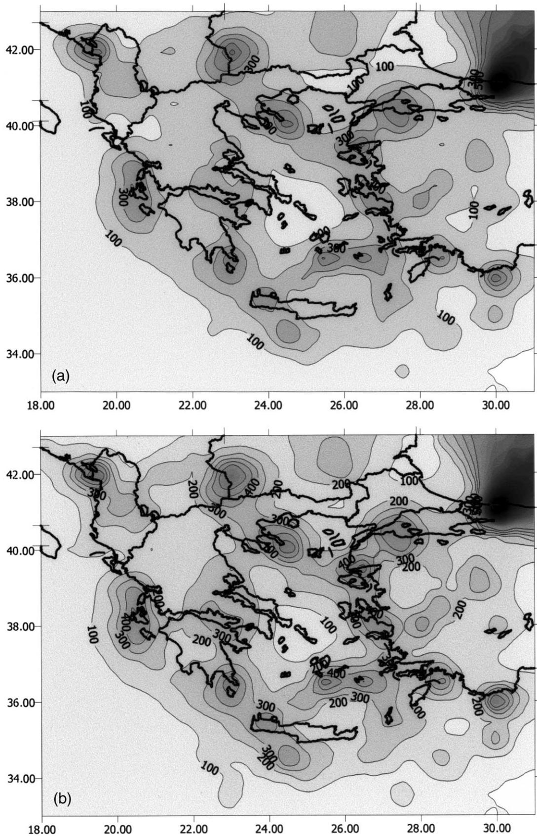
Fig. 7. Seismic hazard maps for Greece using the NTP attenuation relationship for stiff soil sites. Contours are expected maximum p.g.a.  $\text{cm s}^{-2}$  for 50-percentile values using data 1900–1999 with  $M_S \geq 5.5$ : (a) 90% p.n.b.e. during 50-year; (b) 90% p.n.b.e. during 200-year; (c) 70% p.n.b.e. during 50-year; and (d) 90% p.n.b.e. during 50-year using data 1964–1999.
