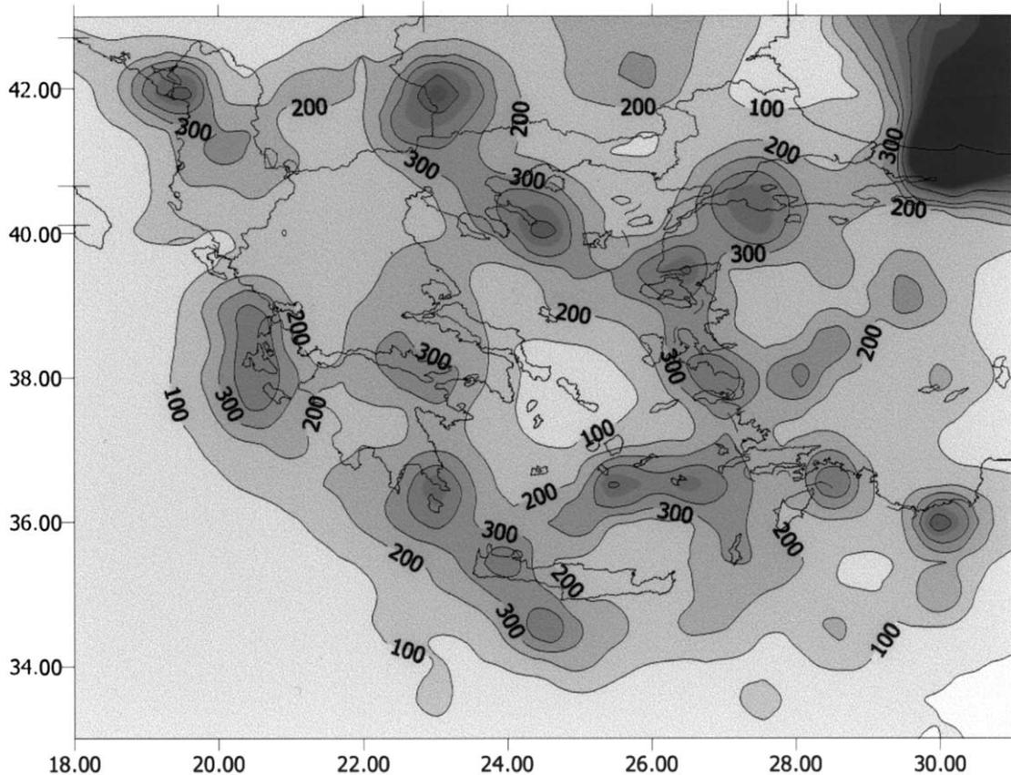
Fig. 6. Seismic hazard map for Greece using the TP attenuation relationship for rock sites. Contours are expected maximum p.g.a.  $\text{cm s}^{-2}$  with 90% p.n.b.e. during 50-year for 50-percentile values using data 1900–1999 with  $M_S \geq 5.5$ .
