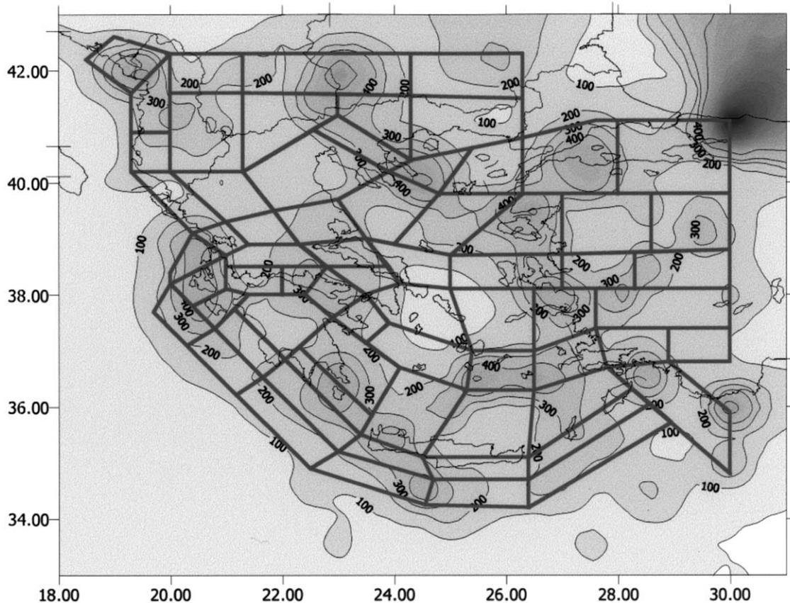
Fig. 8. Seismic hazard map for Greece using the NTP attenuation relationship for stiff soil sites with the 67 Papazachos and Papaioannou seismogenic source zones ([34]) superimposed. Contours are expected maximum p.g.a.  $\text{cm s}^{-2}$  with 90% p.n.b.e. during 50-year for 50-percentile values using data 1900–1999 with  $M_S \geq 5.5$ .
