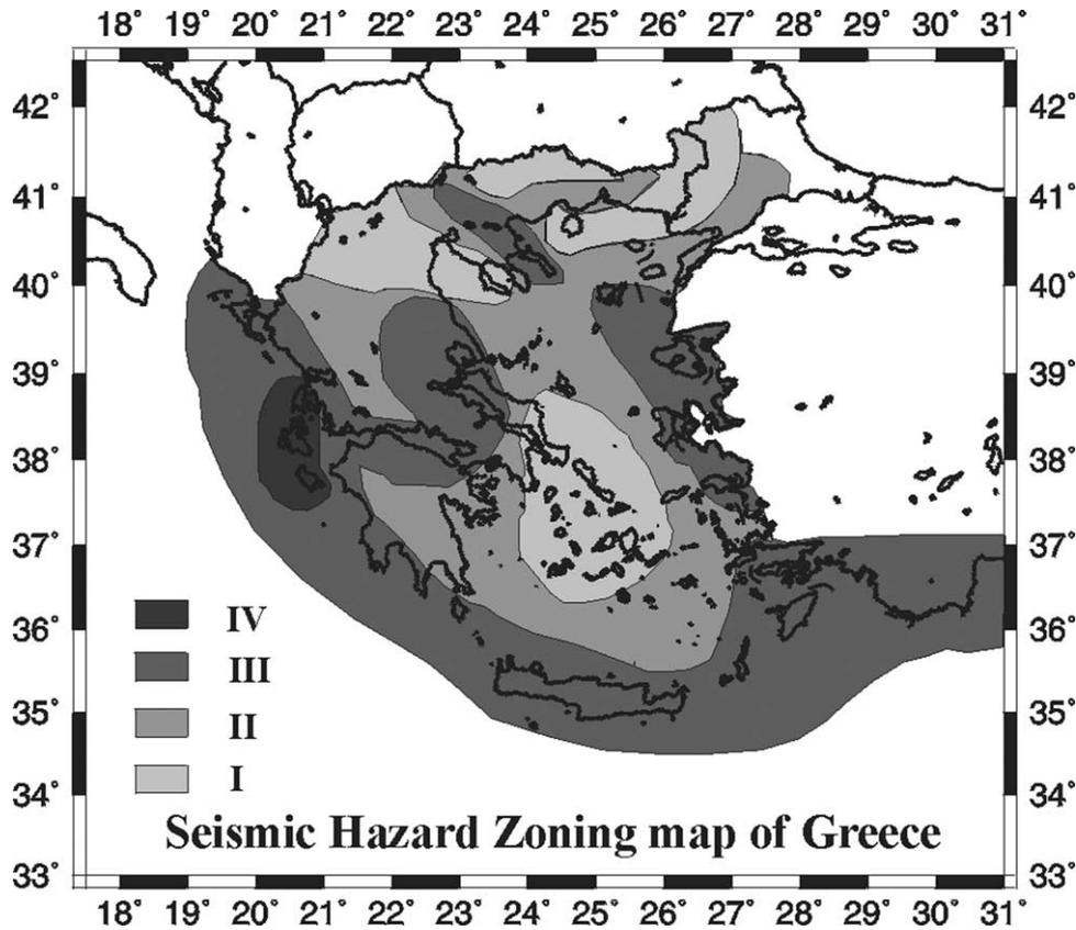
Fig. 1. Seismic hazard zoning map of Greece adapted from the New Greek Seismic Code (NEAK). NEAK addresses average horizontal p.g.a. values (%g) for a mean-return period of 475-year and adopts four zones: Zone I 12%g, Zone II 16%g, Zone III 24%g, Zone IV 36%g.
