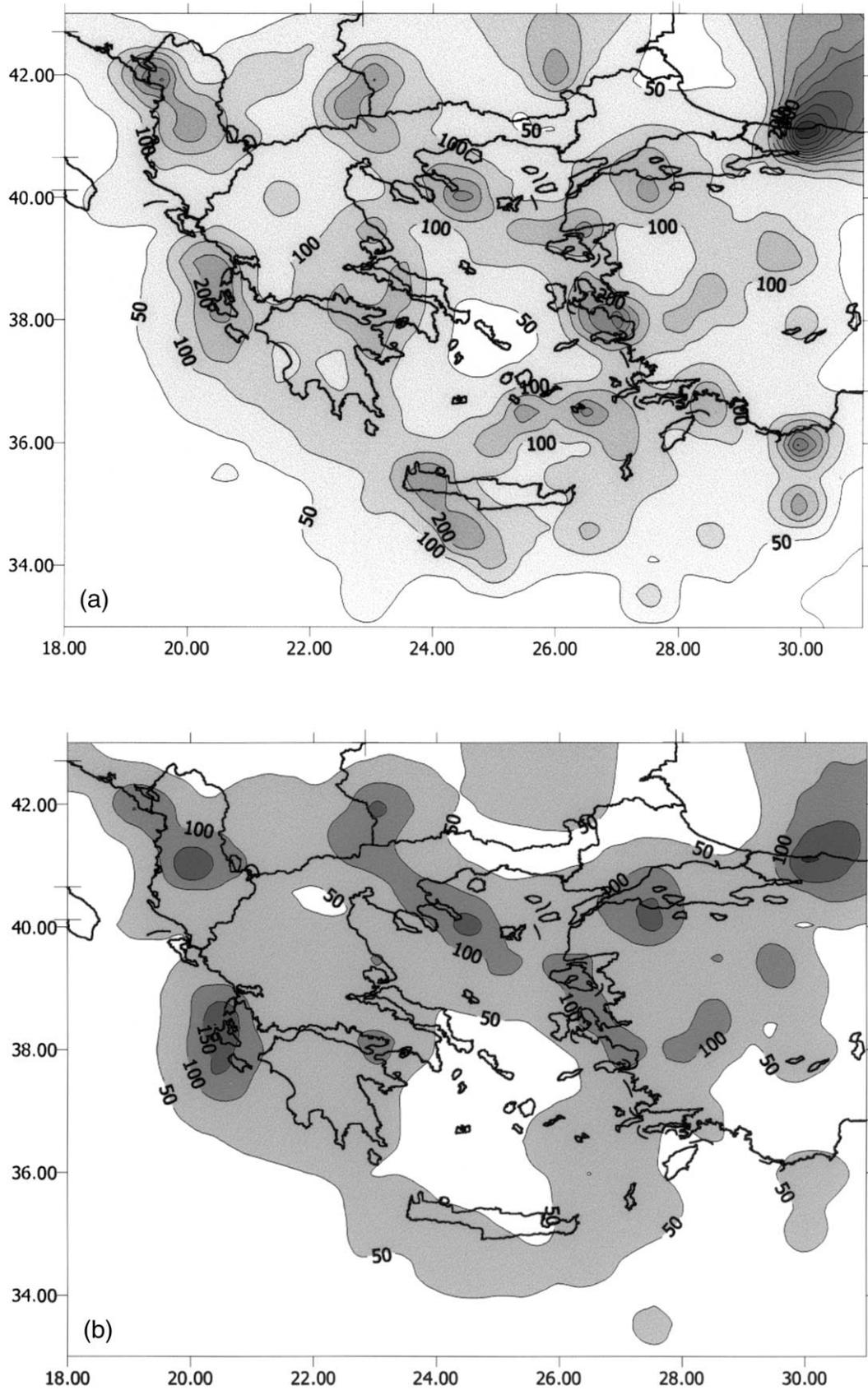
Fig. 5. Seismic hazard maps for Greece using the AM attenuation relationships. Contours are expected maximum p.g.a.  $\text{cm s}^{-2}$  with 90% p.n.b.e. during 50-year. Fifty-percentile values for rock sites using data 1900–1999 with  $M_S \geq 5.5$  are shown, derived from the AM model: (a) without and; (b) with depth control.
