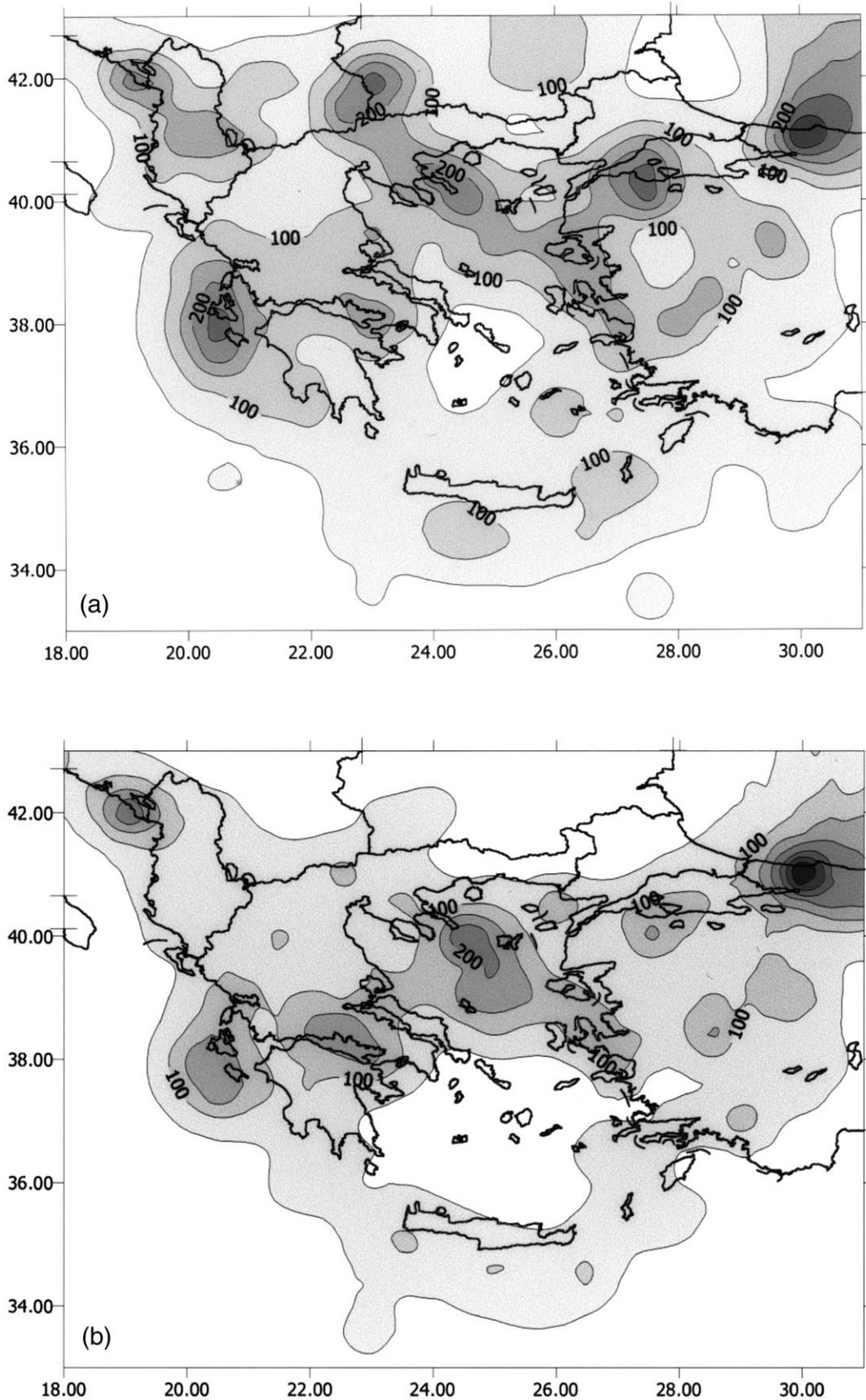
Fig. 4. Seismic hazard maps for Greece using the MB attenuation relationship, illustrating contours of expected maximum p.g.a.  $\text{cm s}^{-2}$  with 70% p.n.b.e. during 50-year: (a) using data 1900–1999 with  $M_S \geq 5.5$ ; (b) using data 1964–1999 with  $M_S \geq 4.0$ .
