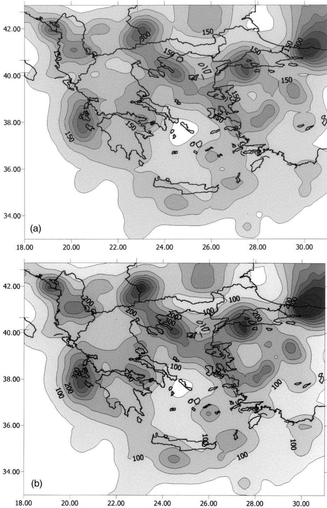
Fig. 3. Seismic hazard maps for Greece using the MB attenuation relationship. Contours are expected maximum p.g.a.s (p.g.a. cm s<sup>-2</sup>) with 90% probability of not being exceeded (p.n.b.e.) during time periods: (a) 50-year; (b) 100-year and (c) 200-year, using data 1900–1999 with  $M_S \geq 5.5$ ; (d) is 90% p.n.b.e. during 50-year using data 1964–1999 with  $M_S \geq 4.0$ .
