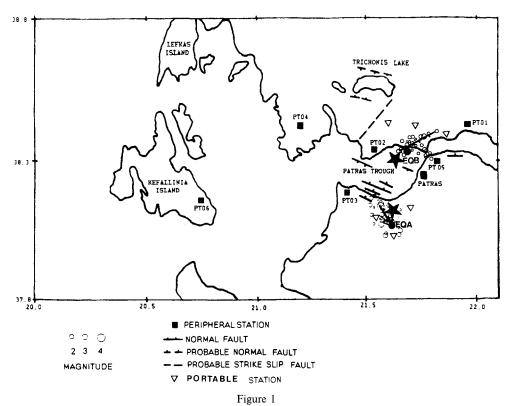
Seismographic stations of Patras Seismological Network used in this study. The star indicates the main shocks. The open circles indicate the aftershock activity. The filled circle indicates the location of the doublet.
