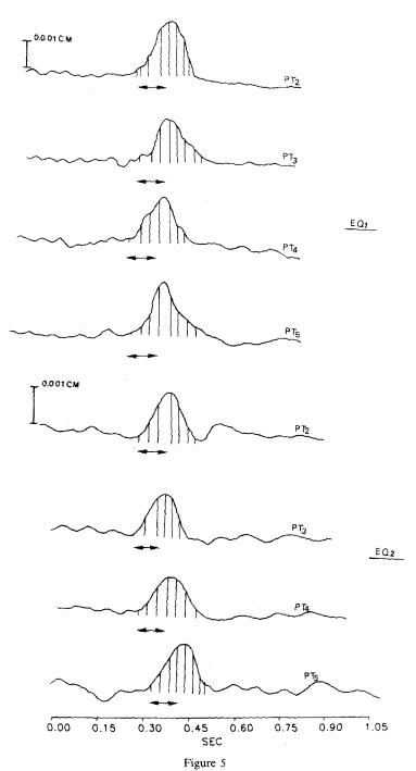
Deconvolved displacement wave forms for EQ1 and EQ2 of the first doublet, at stations PT2, PT3, PT4 and PT5. Shaded region shows the area used for the estimation of the moment. Rise times are indicated by the bars.
